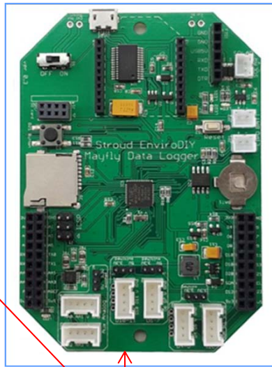
Mayfly data logger board
