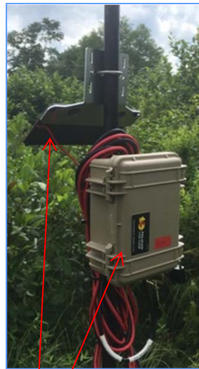
Solar panel and logger box
