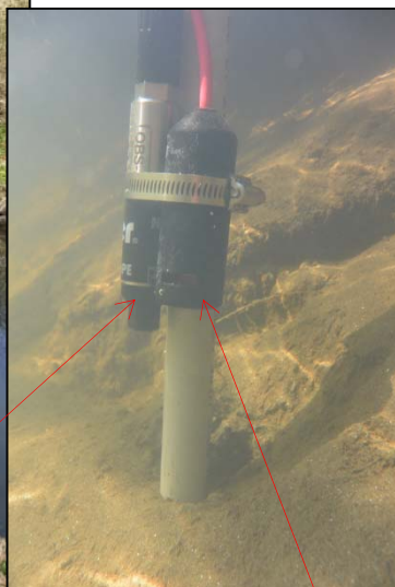
Meter Hydros 21 CTD sensor (formerly Decagon CTD-10)
