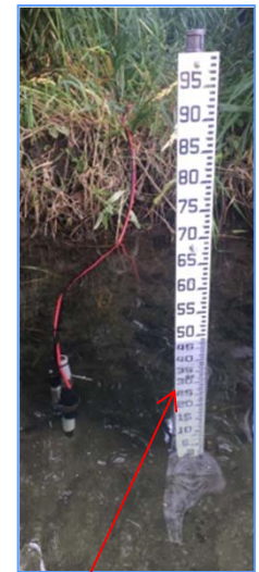
Staff gauge – for on- site reference and use in developing hydrologic rating curves
