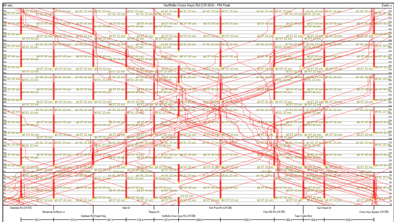
Sample Time-Space Diagram from Tru-Traffic Software – Hurffville-Cross Keys Rd (CR 654) PM Peak Period
