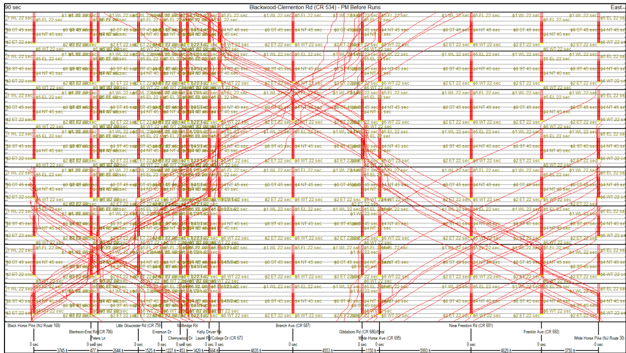
Sample Time-Space Diagram from Tru-Traffic Software – Blackwood-Clementon Rd (CR 534) PM Peak Period
