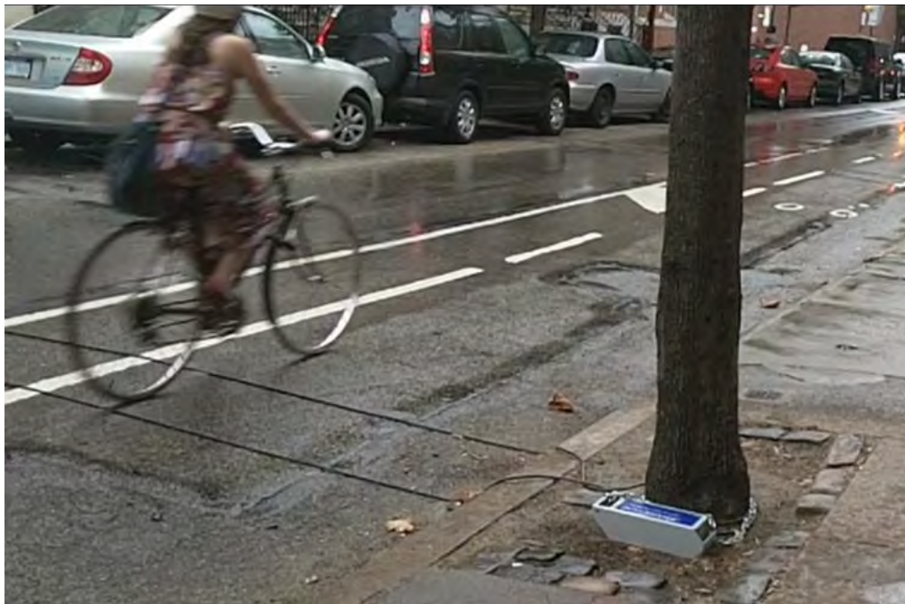
Pneumatic tube bicycle counter in Philadelphia, PA Photo Credit: Bicycle Coalition of Greater Philadelphia
