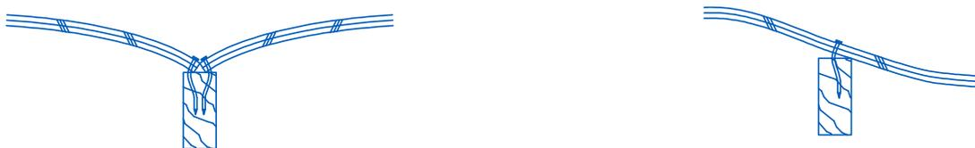
*Figure E.6.1. Sheathing in uplift exerts bending forces on sheathing nails, jamming the nails against the side of the nail hole and providing significant withdrawal resistance even if the hole is enlarged by drying shrinkage. This provides one possible explanation for why test beds built of green lumber appear to have uplift capacities very similar to test beds built of dry lumber, especially for the preferred Foot Positions A and B.*
