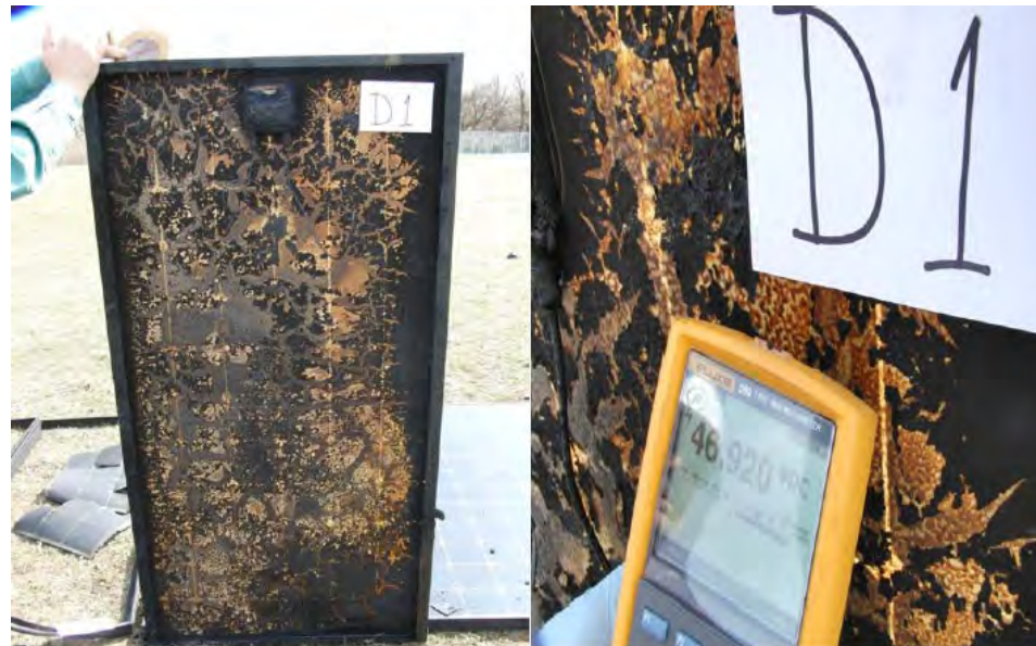
Figure 117 - Module D1 – badly burnt on backside, but functional and producing full voltage
