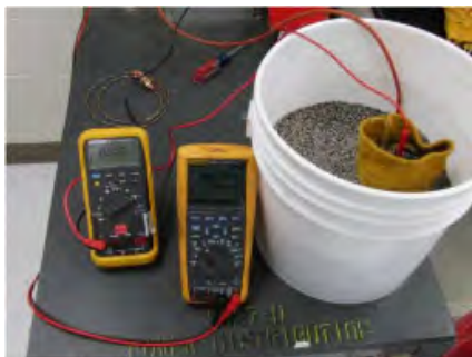
Figure 29 Testing a glove in metal shot
