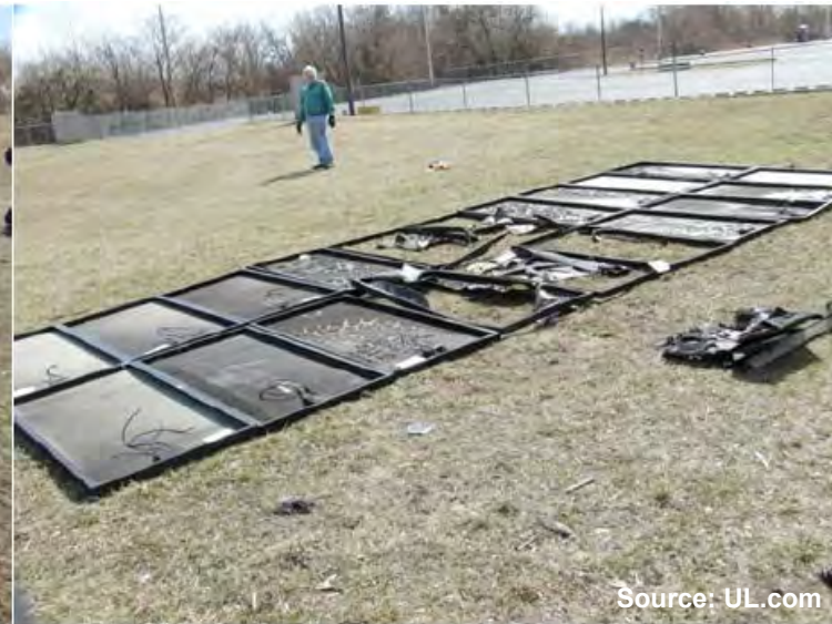
Figure 114 Post fire, back surface
