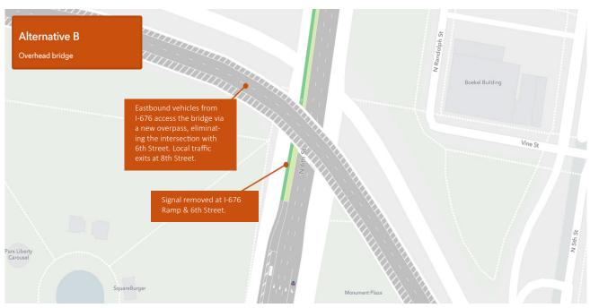
Bridge-bound traffic from 6th Street would still need to use the existing 6th Street on-ramp, but the lower volume would enable a narrowing of that ramp as well as the addition of a signal for pedestrians accessing Monument Plaza.
