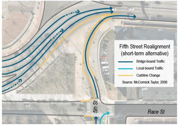
Figure 31: Short-Term McCormick Taylor 5th Street Ramp Realignment
