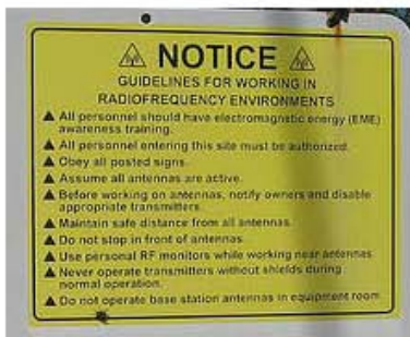
A notice posted at a wireless service facility, warning of electromagnetic radiation.
