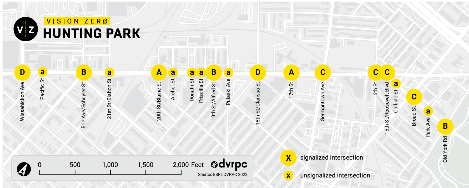
Figure 10: Levels of Service (LOS): AM Peak Hour Existing Conditions
