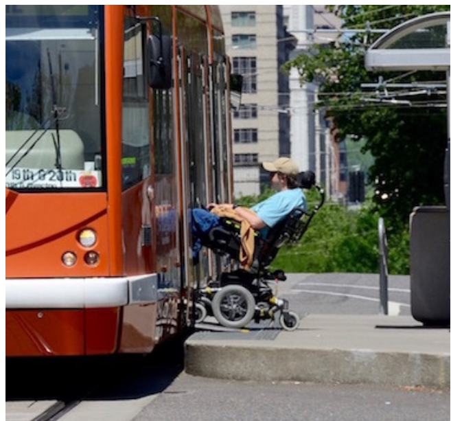
Figure 26 | Portland Streetcar: Automatically deployed ramp Source: Steve Morgan via Wikimedia Commons (CC BY-SA 3.0)
