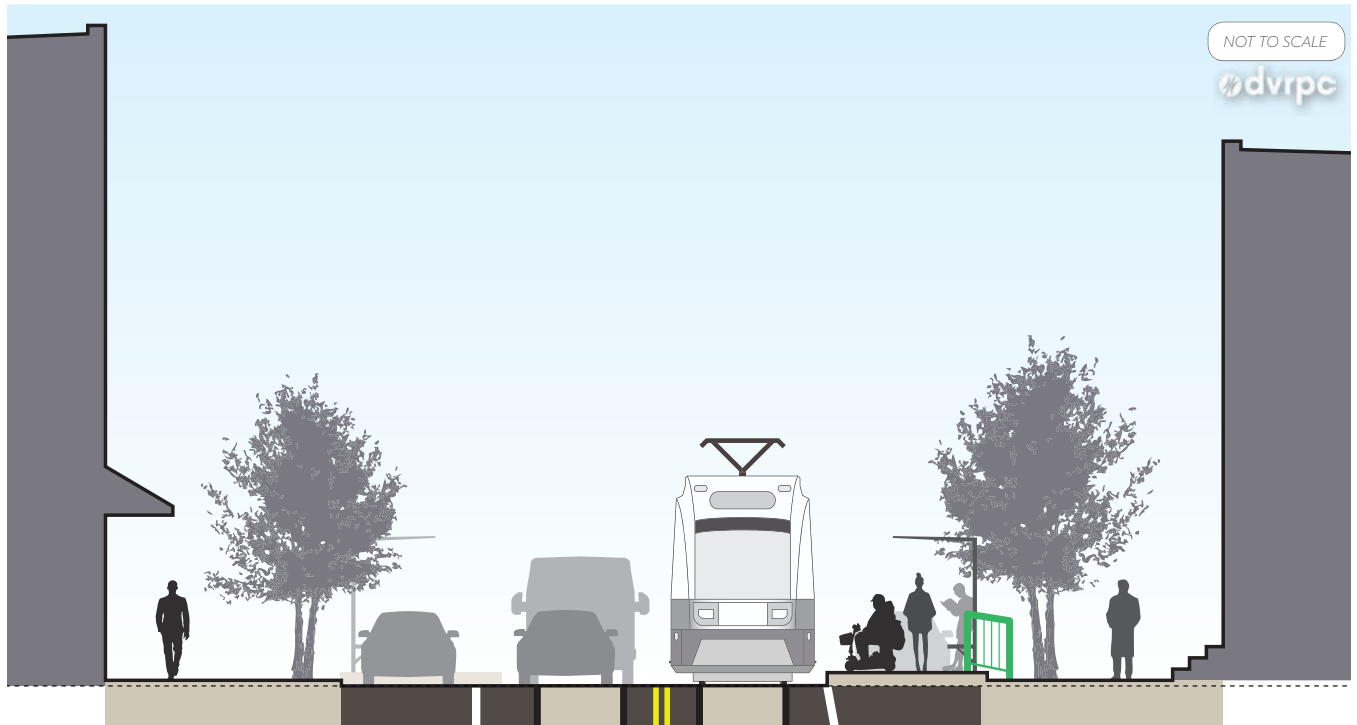
Figure 51 | Curb extension station: Cross-section
