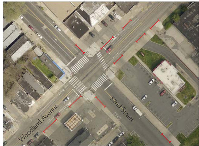
Figure 34 | 52nd Street & Woodland Avenue aerial image with curb cuts shown in red
