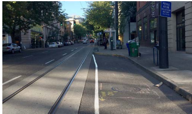
Figure 35 | Portland Streetcar: Shifting lane line
