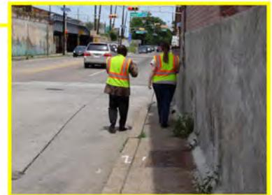
Mt. Ephraim Ave. NB lane extra wide and results in less than adequate sidewalk up to Pine St. and forces pedestrians and wheel chair users into street, this is a hazard and an ADA compliance issue.
