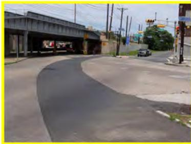
Missing stop bars and crosswalks at Mt. Ephraim Ave. NB, missing pedestrian heads and curb ramps
