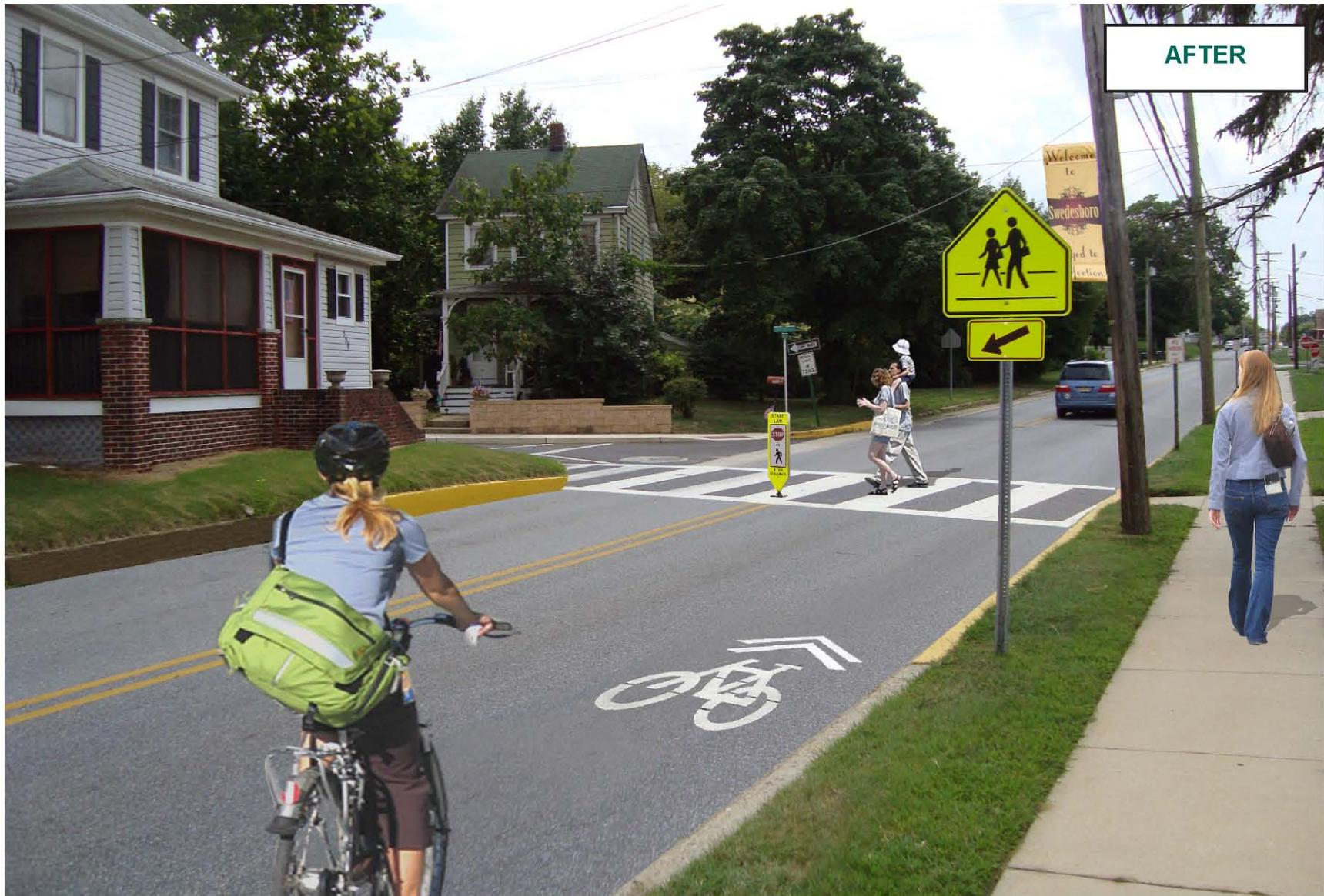
**Figure 11: Auburn Avenue and Poplar Street Simulation** – Photo simulation of proposed improvements near the intersection of Auburn Avenue and Poplar Street. Recommendations include enhanced crosswalk and pedestrian signage, the extension of placemaking elements, and sharrows.
