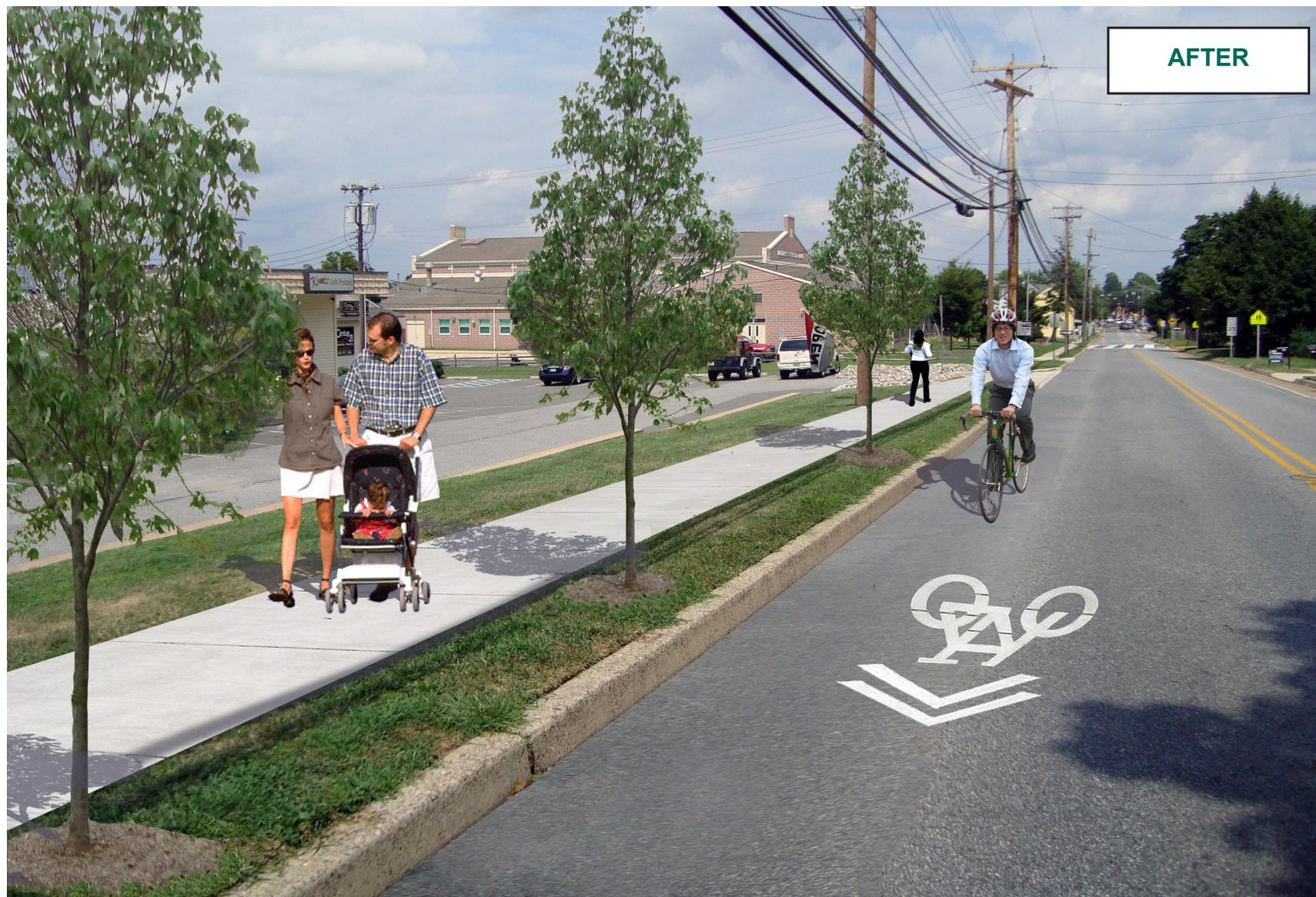
**Figure 8: Area North of Locke Avenue Simulation** – Photo simulation of proposed improvements along Auburn Avenue. A sidewalk and street trees improve the pedestrian environment, while shared lane markings enhance bicycle circulation. (Source: DVRPC)
