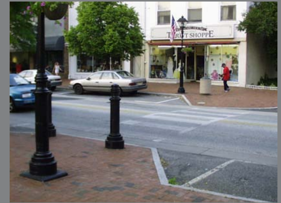
Burlington City, New Jersey's downtown has neckdowns to make crossing the street shorter and safer.
