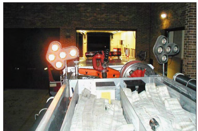
Figure 3.13b—Some department equip their fire apparatus with flashing arrows.
