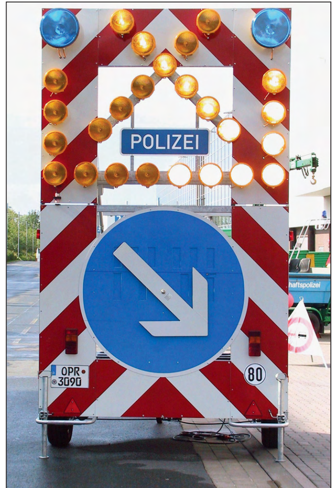
Figure 3.31—This large arrow board trailer is towed by German police vehicles.
