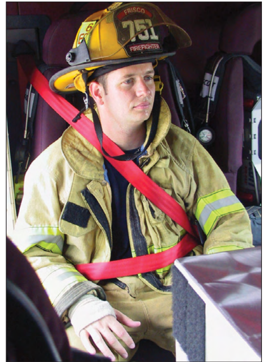
Figure 3.21—NFPA 1901 requires seat restraints to be red.
