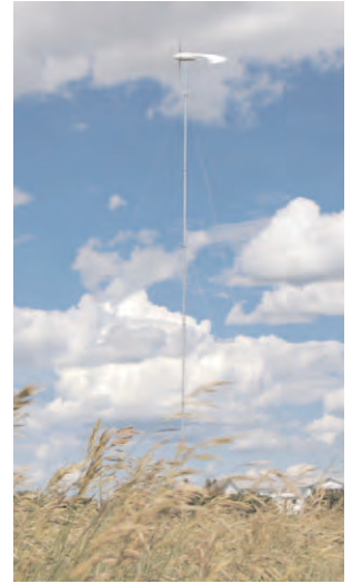
Windward Engineering 4.25kW turbine
