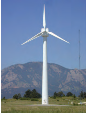
Northern Power 100kW turbine
