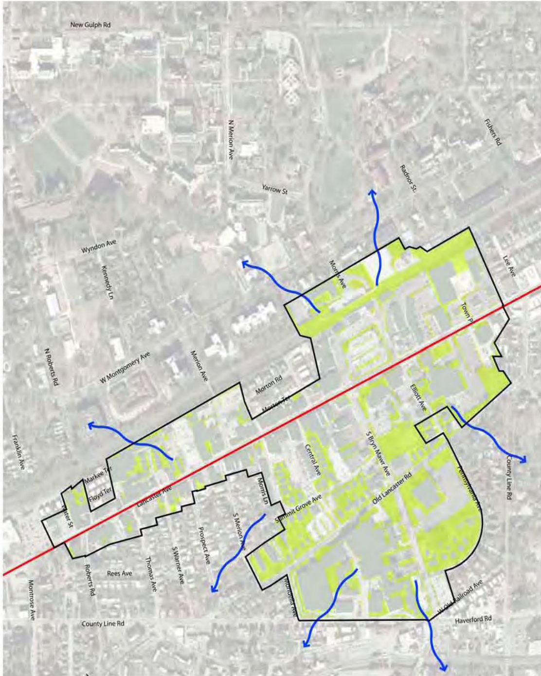
Figure 6: Existing Surface Drainage and Pervious Areas
