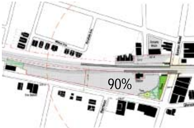
figure 4.1.3 Existing impervious surfaces and pervious green surfaces. These are under utilized areas that have limited activity generated. 90% of the core area is impervious surfaces or SEPTA rail right-of-way.
