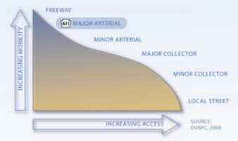
Roadways are classified according to their function, ranging from freeway to local street. A limited-access freeway has access points only at interchanges. No driveways are found on these facilities. This roadway design provides the greatest levels of mobility possible. Conversely, local streets may have many driveways, as mobility on local streets is of secondary importance to providing access to abutting commercial and residential properties.
