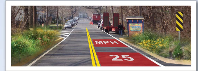
The visualization above illustrates a potential traffic calming and gateway treatment on Elizabeth Street.
