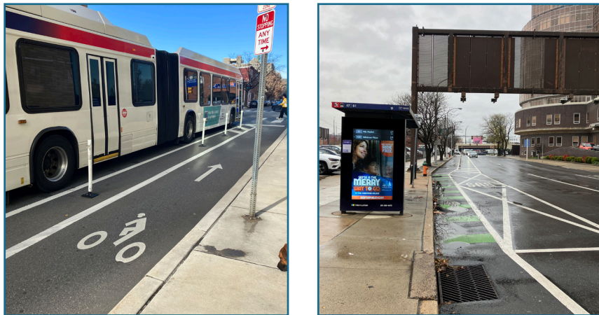
Figure 7: Inability to Curb, Bike Lane Present
