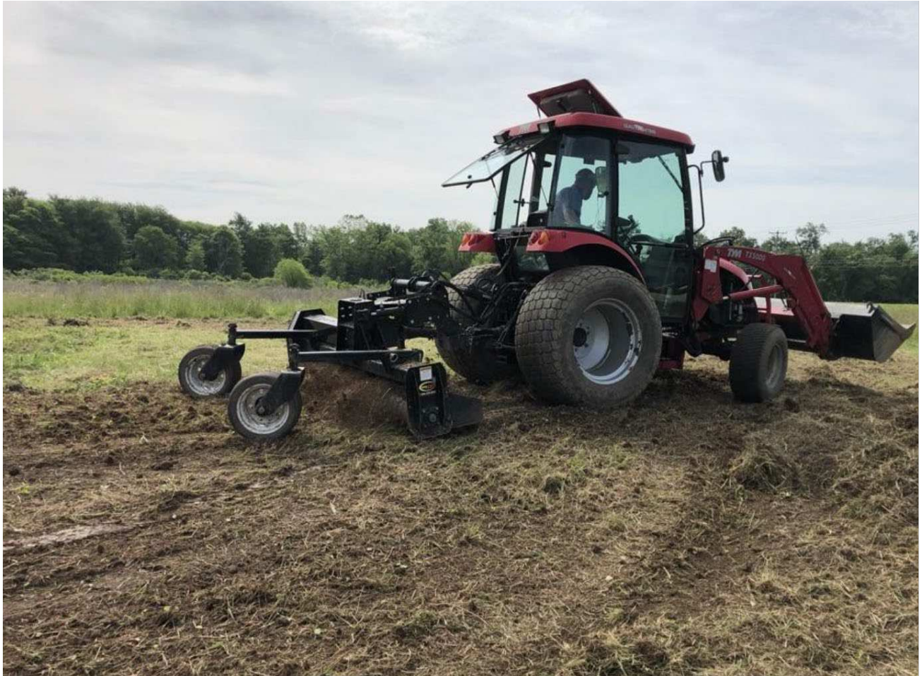
Harley Rake used for the preparation of the soil prior to planting
