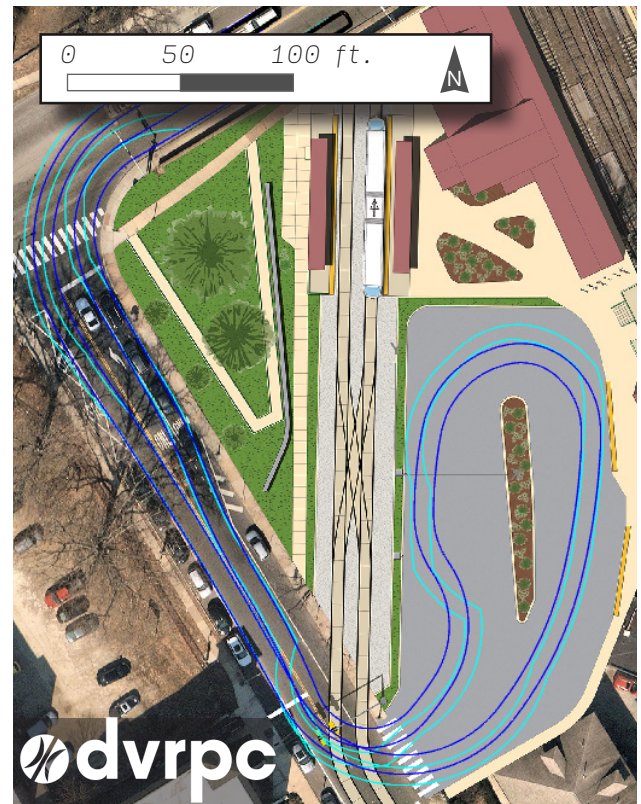
Figure 30: Illustrative turn template created with AutoTURN, southbound bus terminal entry. (DVRPC and Nearmap, 2021)
