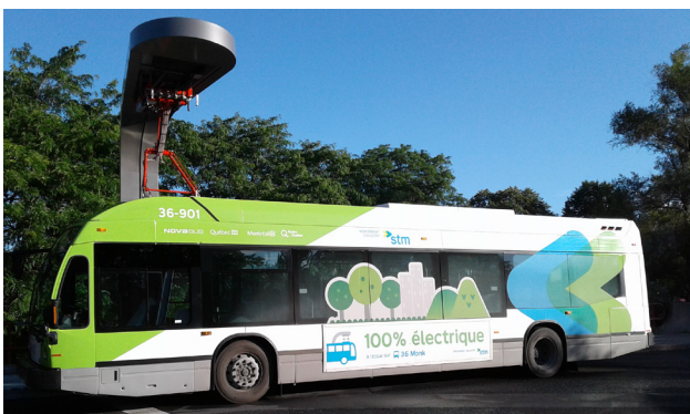
Figure 31: Battery-electric bus charging station from the Société de transport de Montréal. This overhead electric charging station in Montreal acts as one of many options to charge battery-electric buses. (Wikimedia Commons, 2017)
