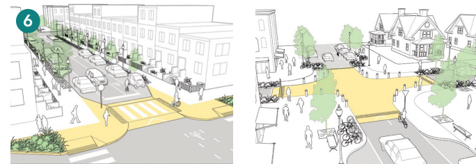
Raised crosswalks (left) and intersections (right) are two types of vertical speed control elements that reinforce slow speeds and encourage motorists to yield to pedestrians at the crosswalk.
