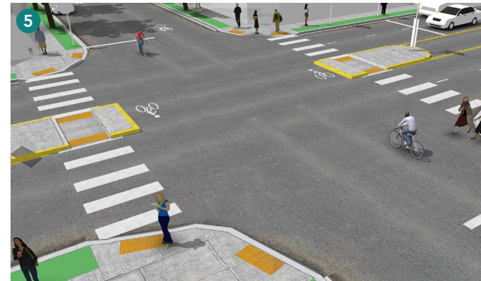
Pedestrian islands allow pedestrians to cross one direction of traffic at a time and help pedestrians feel less exposed at challenging intersections.
