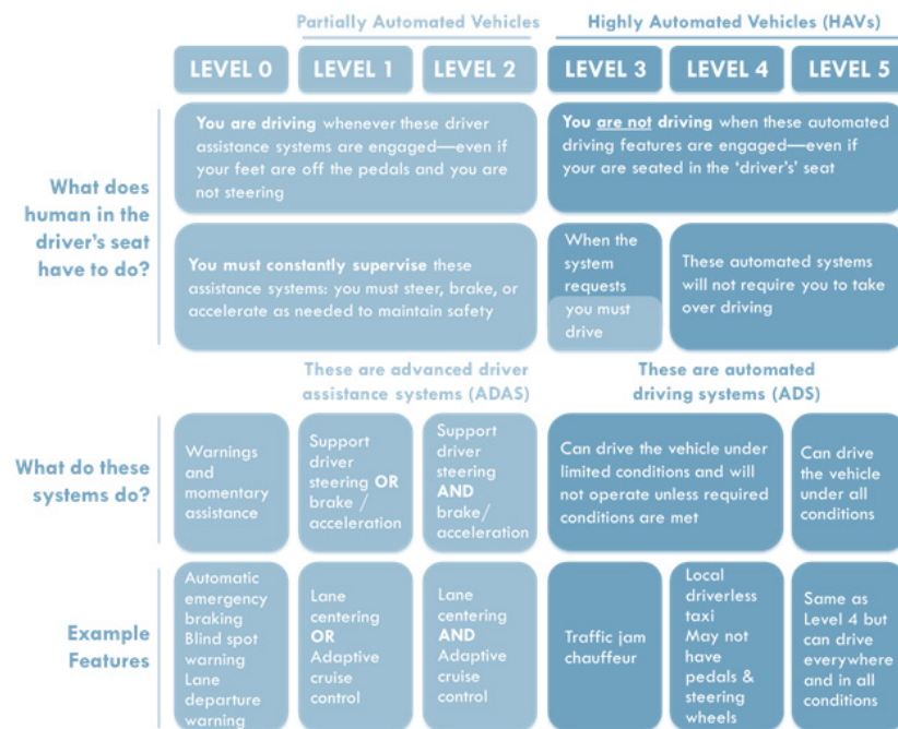
Figure 30: VEHICLE AUTOMATION LEVELS
