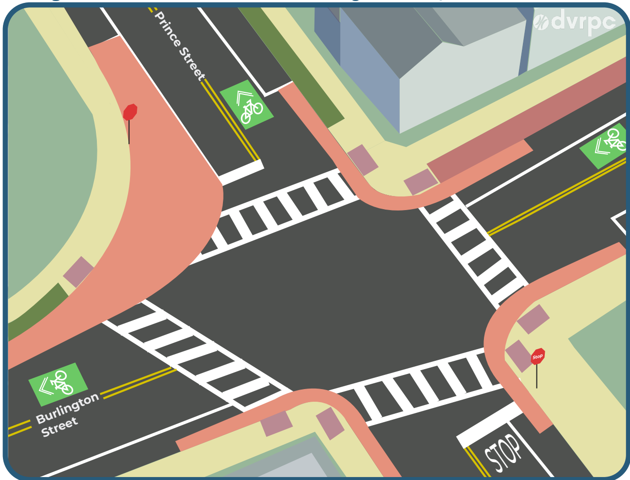
Figure 25 Intersection of Prince Street & Burlington Street: Quick Build Treatments
