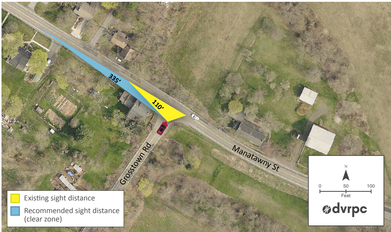
FIGURE C-2: GROSSTOWN RD & MANATAWNY ST SIGHT DISTANCE DIAGRAM
