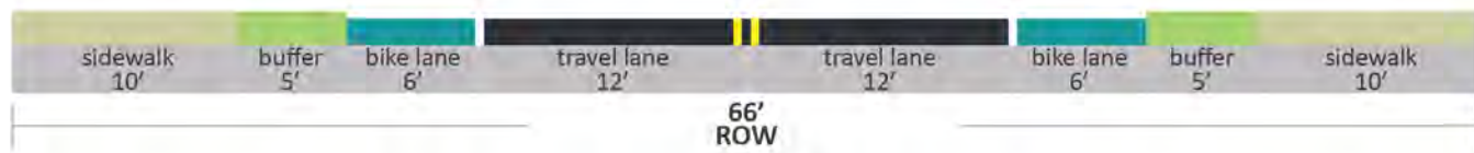
Figure 21: Minor Collector (Maintain)
