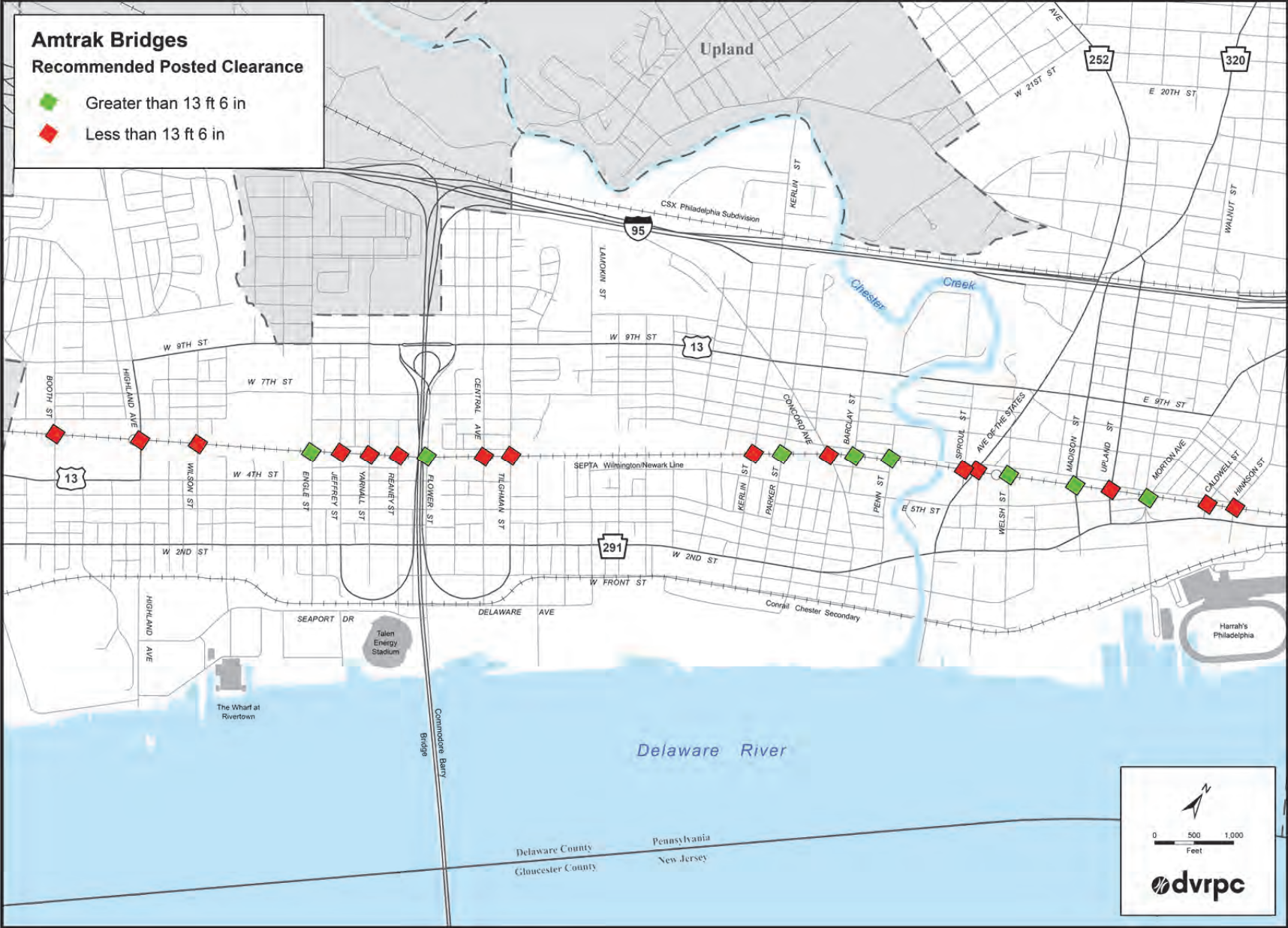
Figure 6: Amtrak Bridge Clearance
