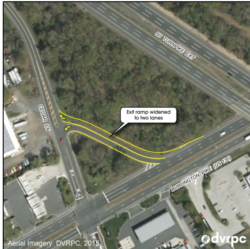
Figure 31: Exit Ramp from US 130 to Cedar Lane (CR 659)
