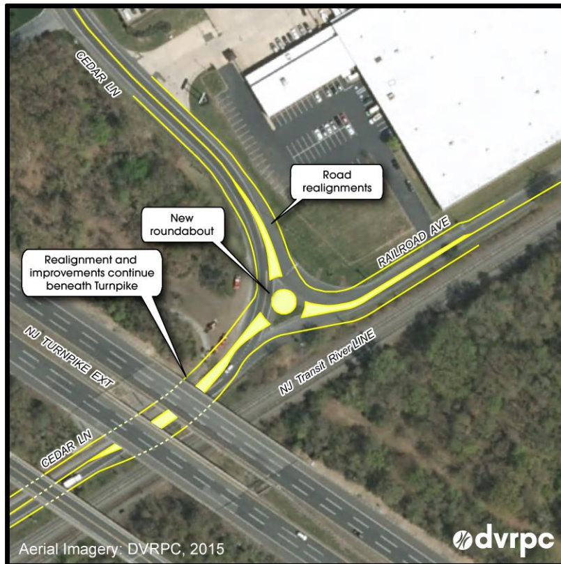
Figure 29: Cedar Lane (CR 659) & Railroad Avenue Roundabout
