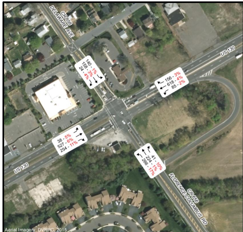
Figure 14: US 130 & CR 656 Florence-Columbus Road Turning Movement Counts – PM Peak Period (4:30 PM to 5:30 PM)
