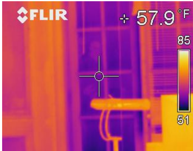
Figure 4: Window Glazing Thermal Performance
