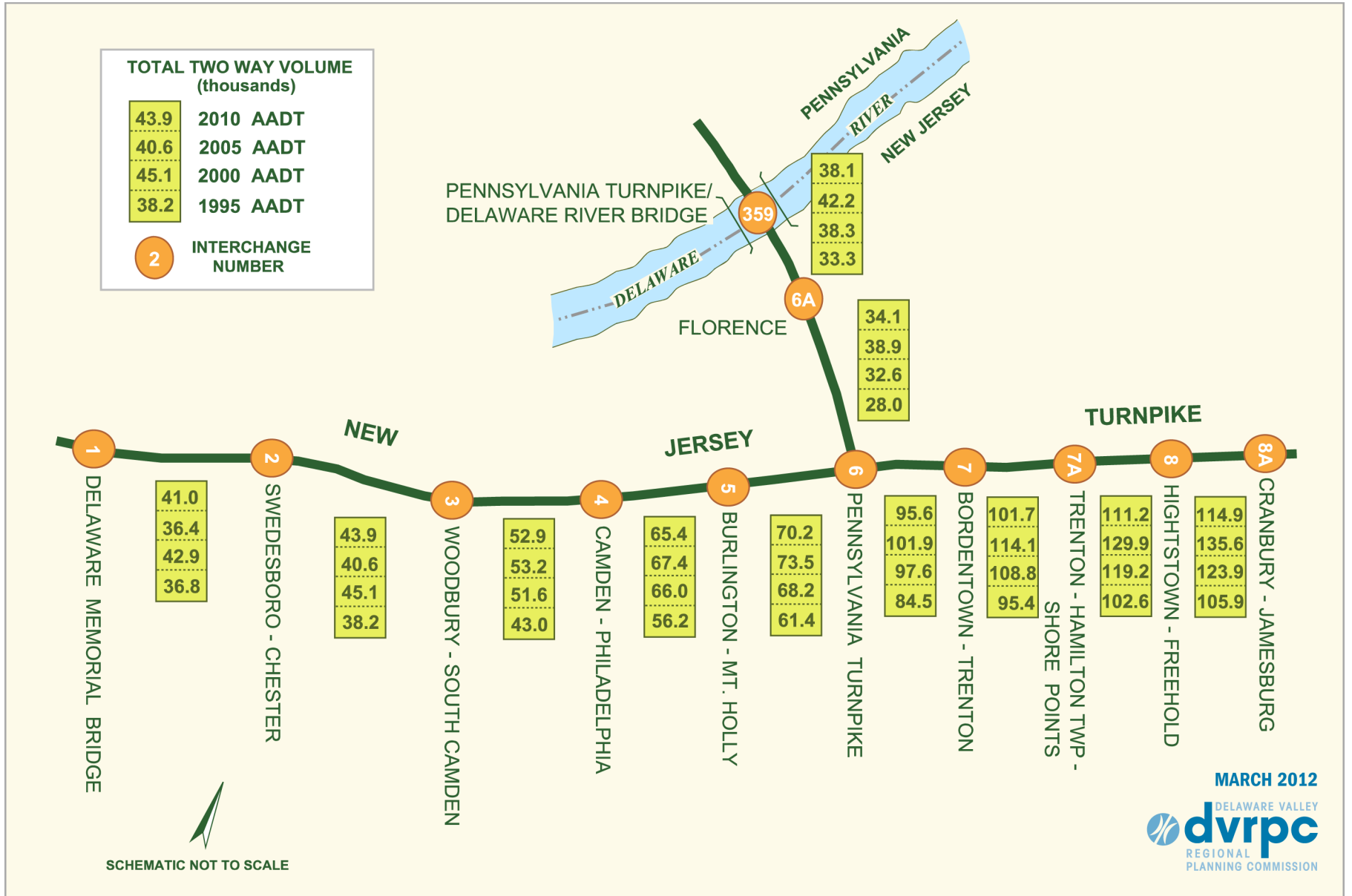
Figure 31: New Jersey Turnpike
