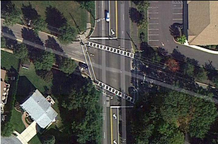
Aerial view of intersection illustrating skewed alignment
