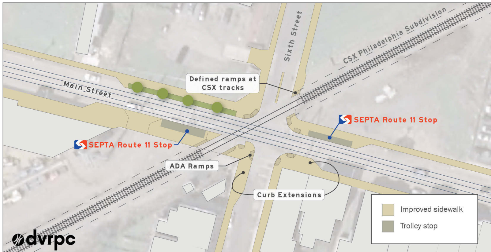
Figure 5: Sidewalk improvements at Main and Sixth streets
