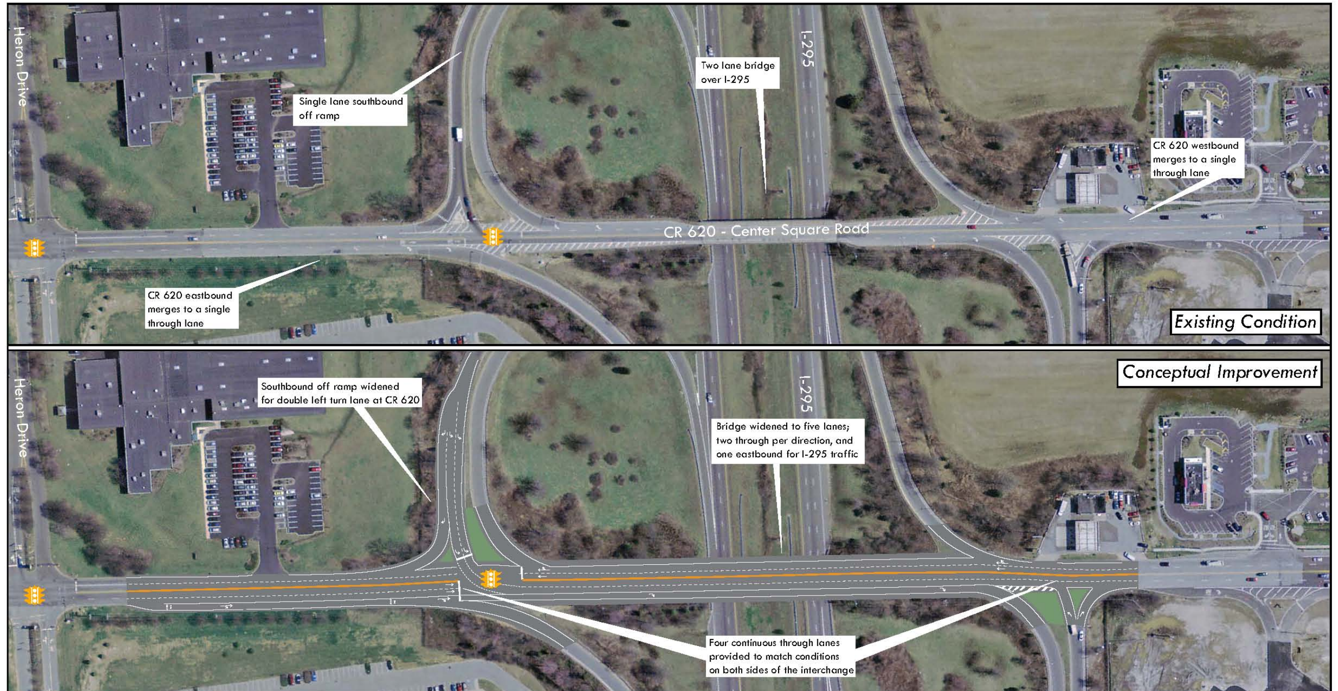
Figure 22: I-295 / CR 620 Interchange Improvement Concept
