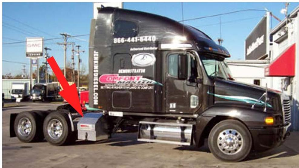
*A Comfort Master APU attached to the underside of the truck between the cab and wheel base. (Source: [www.comfortmaster.com](http://www.comfortmaster.com))*
