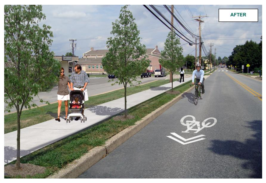
Figure 8: Area North of Locke Avenue Simulation – Photo simulation of proposed improvements along Auburn Avenue. A sidewalk and street trees improve the pedestrian environment, while shared lane markings enhance bicycle circulation. (Source: DVRPC)
