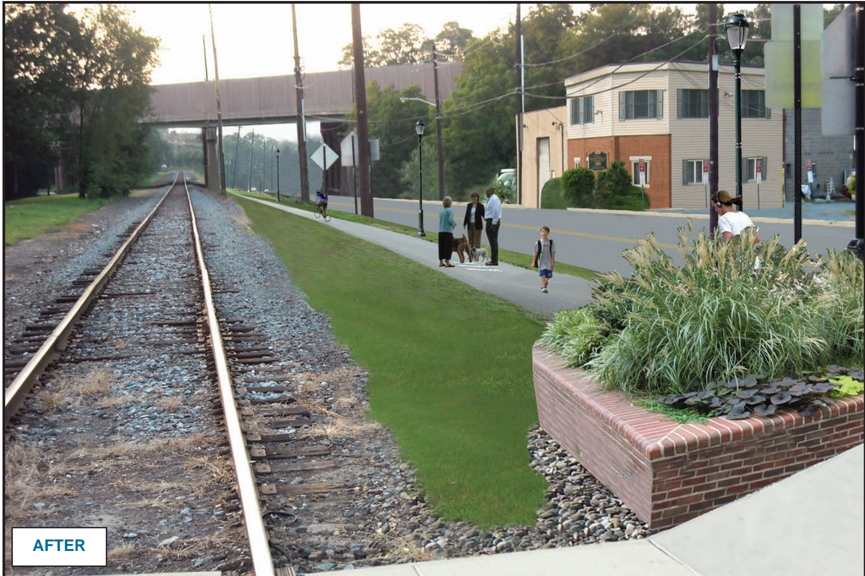
FIGURE 27: Vicinity of Clements Bridge Road, Looking West – Simulation. This image is a photo-simulation of the recommended improvements applied to the location shown on the left. Major improvements include the lane re-striping on East Atlantic Avenue and the installation of a multi-use trail along the railway. Source: DVRPC
