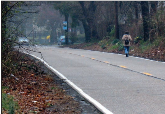
Segments of the corridor lack sidewalks. Coupled with narrow shoulders and sloping berms along the roadside, pedestrians are often forced to walk in the cartway. Source: DVRPC
