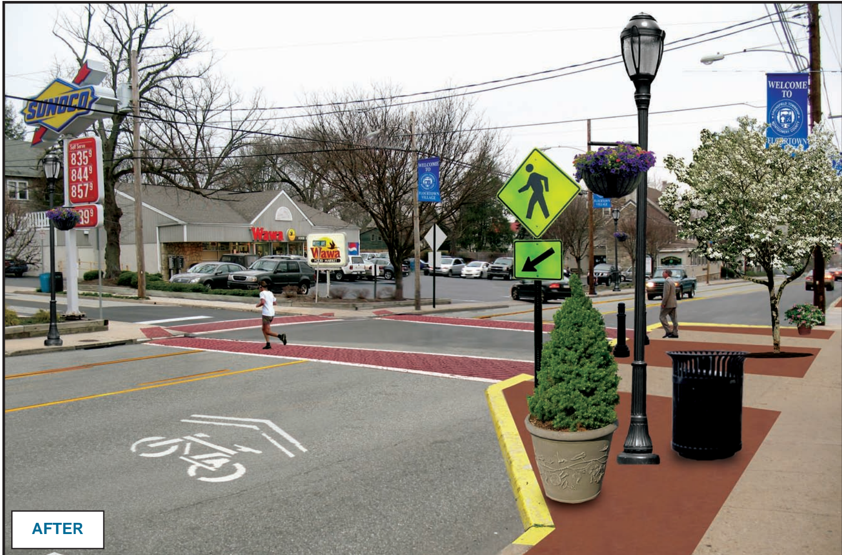
FIGURE 14: Vicinity of Montgomery Avenue – Simulation. This image is a photo-simulation of the recommended improvements applied to the location shown on the left. Major improvements include the new crosswalk at the unsignalized Weiss Road intersection, the three-lane cross-section, shared-lane markings, dedicated parking lane, enhanced crosswalks, streetscaping, and curb extension. Source: DVRPC
