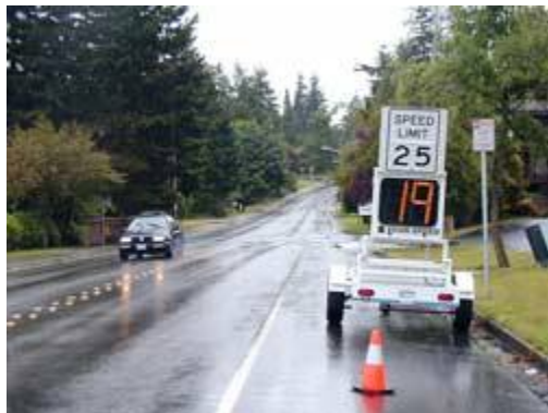
A trailer-mounted Driver Feedback Sign Photo by: http://www.ci.bellevue.wa.us/traffic_calming_overview.htm City of Bellevue, WA
