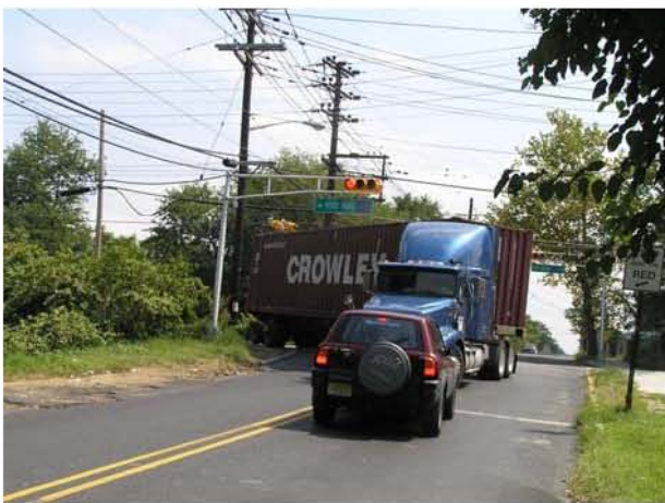
A truck turns into the opposing lane of traffic to make a turn at 36 th Street and River Road along the Crowley American Transport at Petty's Island Connector
