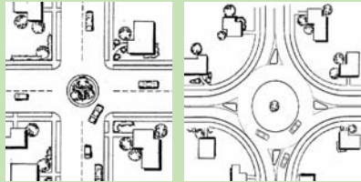
Traffic circle (left) and roundabout (right)
