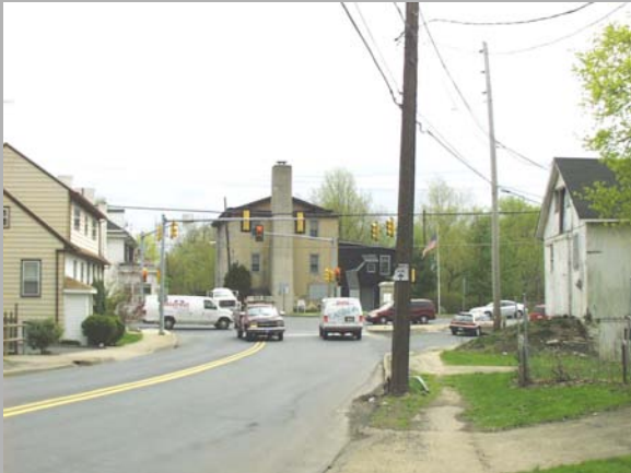
Cars sometimes have difficulty staying in lane when making the tight right-hand turn. An easy solution may be to move the stop line back for cars waiting at a red light along Route 513 South, so there will be less of a chance of an accident.
