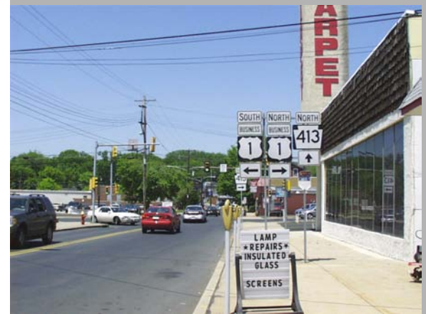
Consolidate street signage to widen usable sidewalk space as well as prevent clutter of signs.
