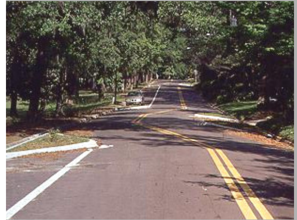
Above is an example of a chicane with a parking lane. Source: http://www.trafficcalming.org .
