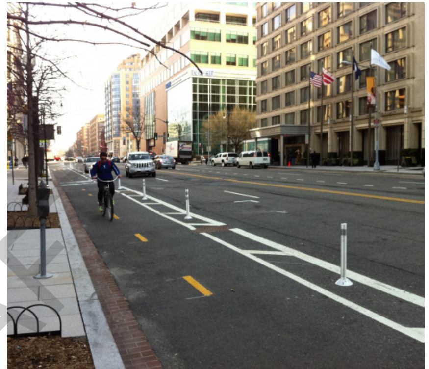
A protected bicycle lane including a painted buffer and vertical flexposts. Source: Megan Kanagy, District Department of Transportation.
