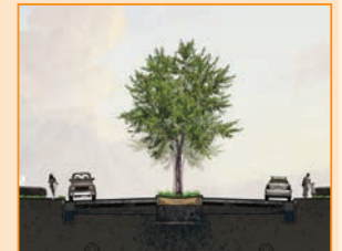
Cross section of a raised median with landscaping and an underground drainage system. Source: Philadelphia Water Department
