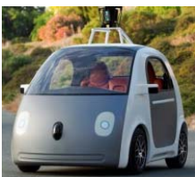
Google's latest self-driving vehicle does not contain a steering wheel or brake pedal. Source: Google
