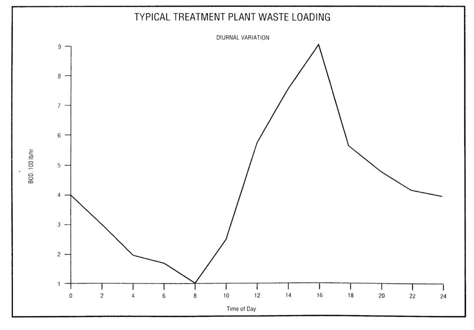
Figure 2. Variation in influent wastewater strength over 24 hours for a typical treatment plant.
