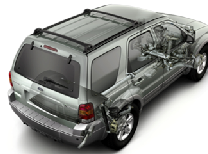
Cutaway Ford Escape showing hybrid components. Source: Green Car Congress.
