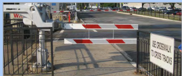
Pedestrian gate with “gate skirt” being tested at the Aberdeen-Matawan Train Station. Image: The RBA Group
