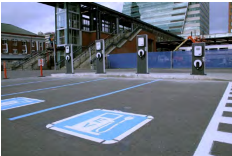
Figure 14. EV Parking Stall with D9-11b (Alternate) Symbol on Pavement
