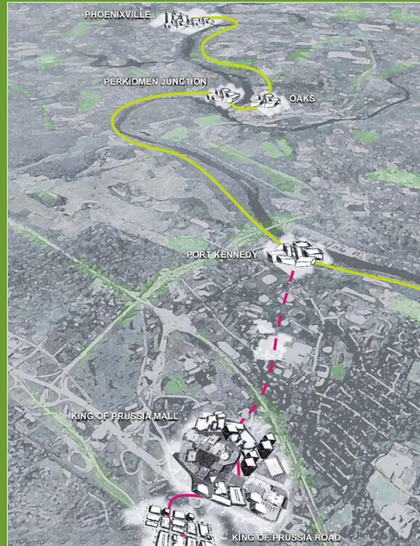
Foreground: Route 100 extension stations at King of Prussia Rd. and King of Prussia Mall. Dotted line indicates possible second phase connection at Valley Forge. Background: proposed R6 extension to Phoenixville, with intermediate stations.
