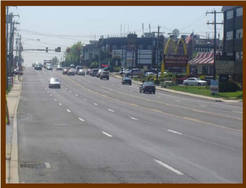
Traffic signal heads are not aligned with lanes at the eastbound approach of the Hulmeville Road intersection
