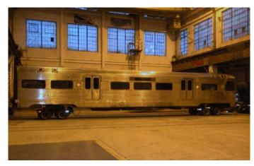
A PATCO rail vehicle undergoing reconstruction. Seventy-five of PATCO's 121 vehicles date from the opening of the line in 1969. Each car will be fully rebuilt to modern standards, while revising the metal shell.
